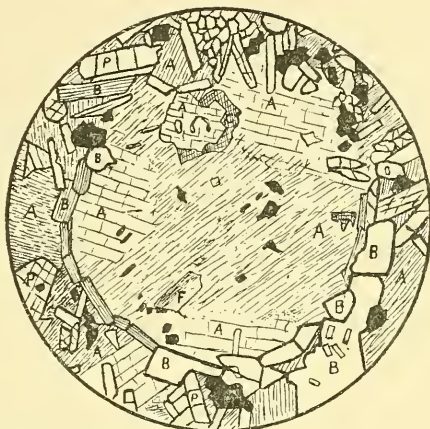
Fig. 3. Micro-drawing of a spheroid. Lettering as in fig. 2. In addition C is calcite, F is feldspar. Actual field 3.5mm.
