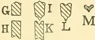
Figure 2.—Sectional diagrams, showing the elasto-viscous deformations of exuded cylinders of the charge C , Fig. 1, external pressure being zero.
