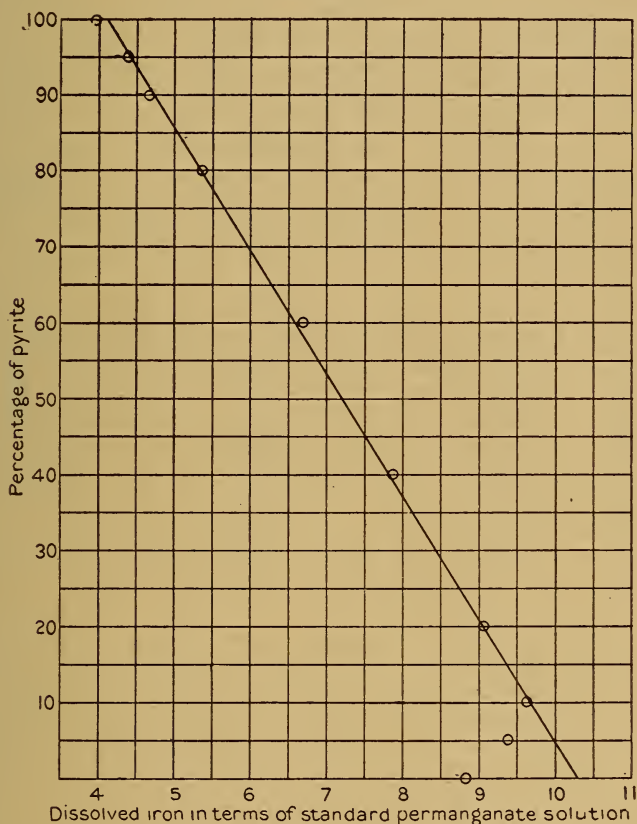
FIG. 2. Stokes' results on iron dissolved ( x-a ) from pyrite-marcasite mixtures by a standard ferric sulphate solution. The values for x are calculated from Stokes' published values for p , the percentage of sulphur oxidized.
