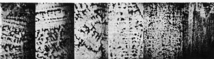
No. 4.—Hardened and tempered from the left. Bessemer Metal in Cast Ingots.
