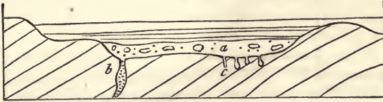
Junction of unconformable strata near Mons, in Belgium.
