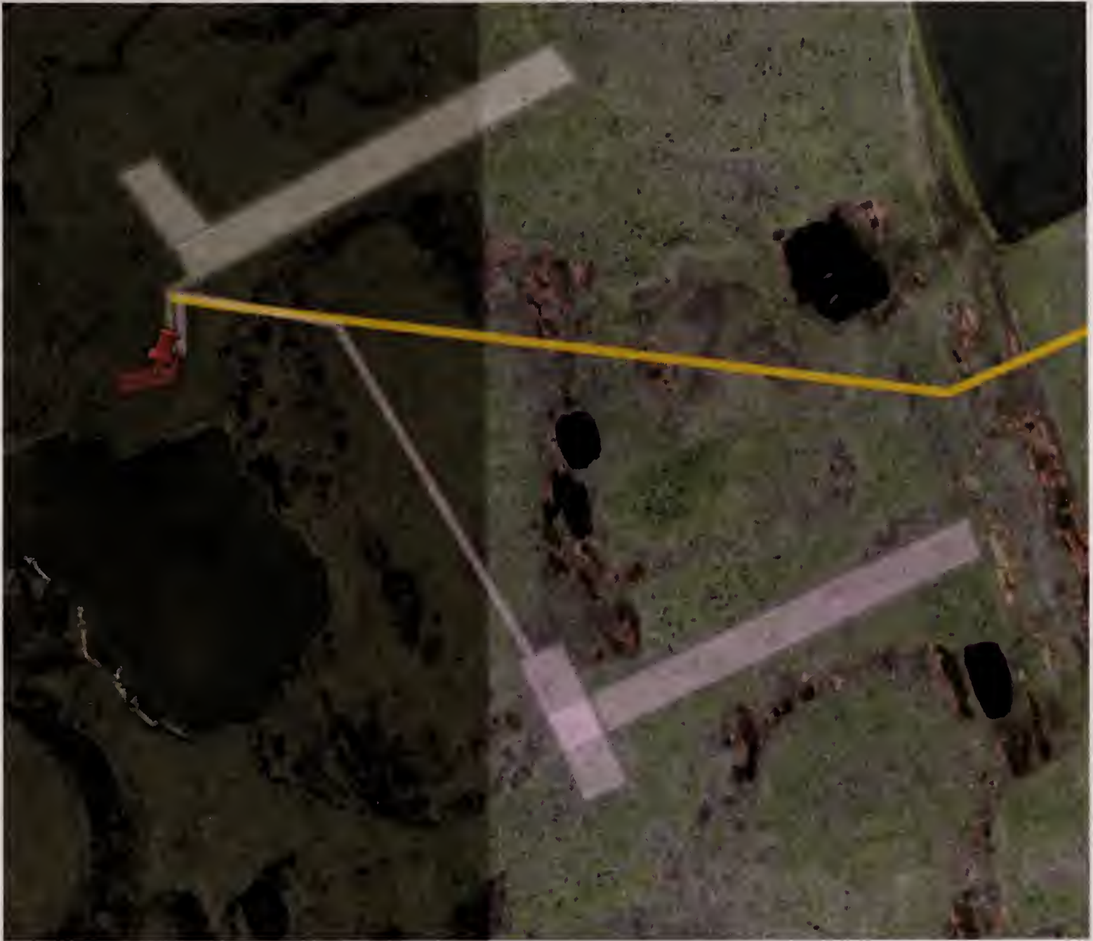
Figure 1. Proposed alternate location (top, gray) for the airstrip for a roadless alternative which reduces the overall footprint; pipeline (yellow/orange) as in Alternative B for separation. Original airstrip (bottom, pink) for Alternative D shown for comparison.
