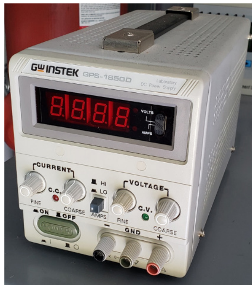
Figure 22. External power supply used for fuel cell start-up
