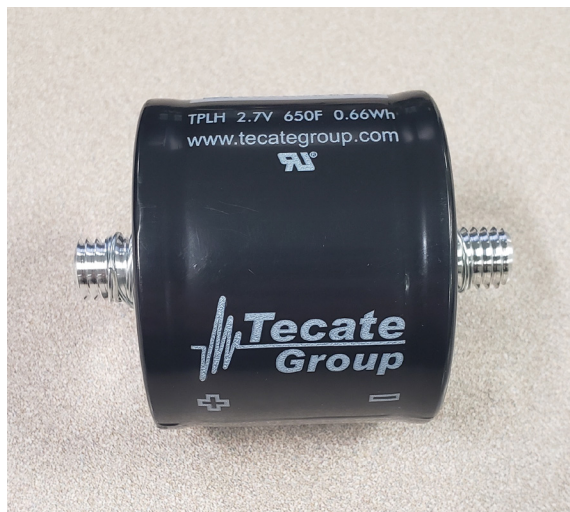
Figure 18. Tecate Group 2.7 volt 650 Farad ultracapacitor
