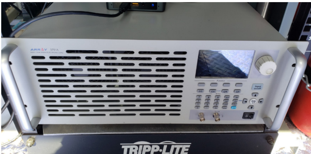
Figure 28. Array 2 kilo-watt DC programmable electronic load
