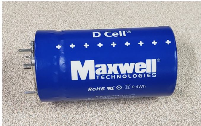
Figure 20. Maxwell Technologies 2.7 volt 350 Farad D Cell ultracapacitor
