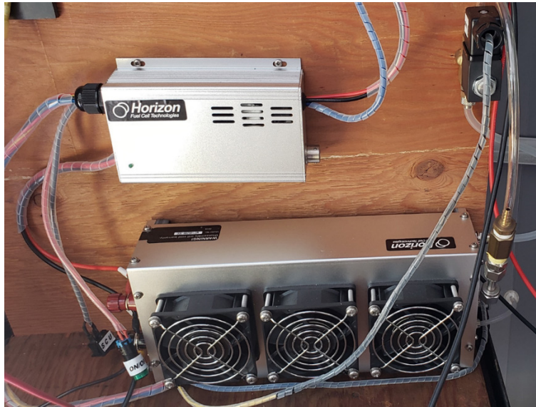
Figure 16. Horizon 300 watt PEM fuel cell and fuel cell controller
