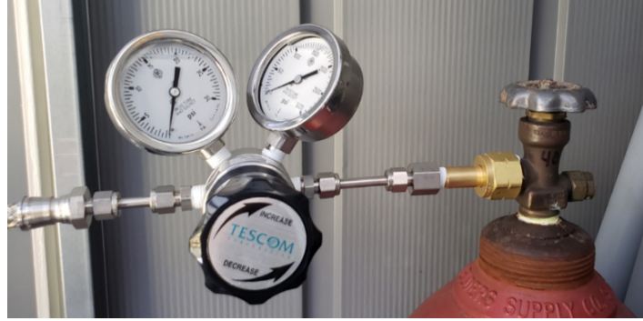
Figure 15. Regulator used to bring tank pressure to 0.5 bar for fuel cell use
