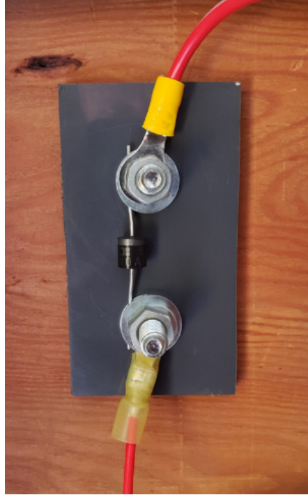
Figure 24. Diode used to restrict current flow from ultracapacitors back into the fuel cell
