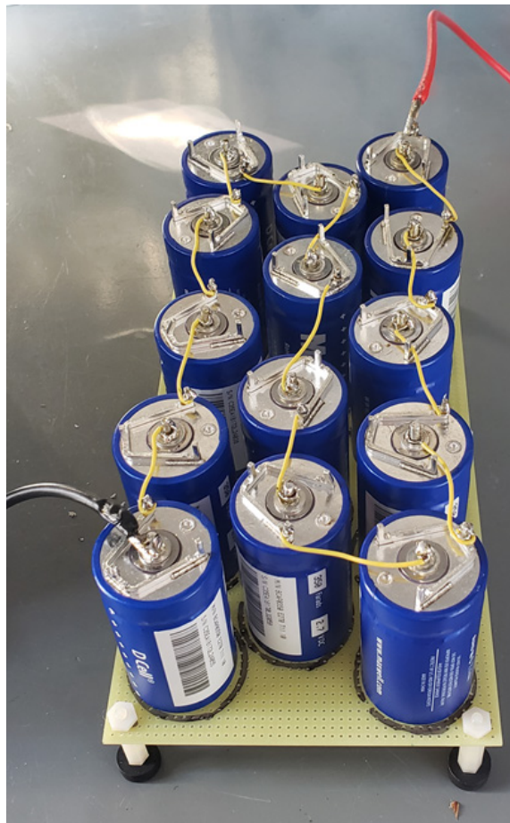
Figure 21. 14 Maxwell Technologies ultracapacitors in series
