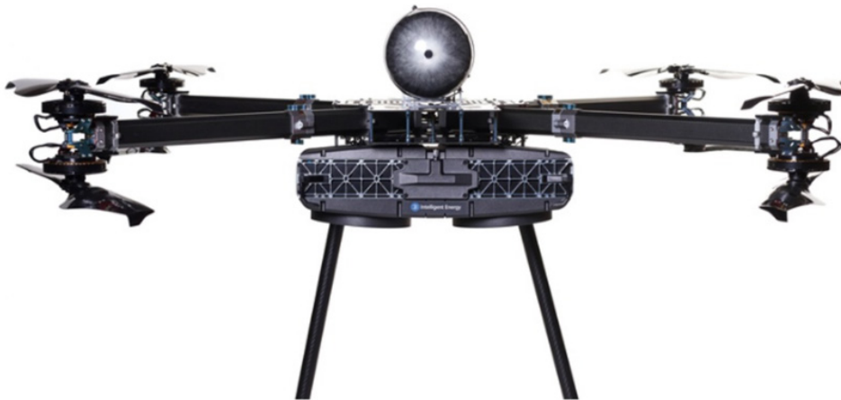
Figure 8. Intelligent Energy's fuel cell power module mounted on a UAS. Source: [23].
