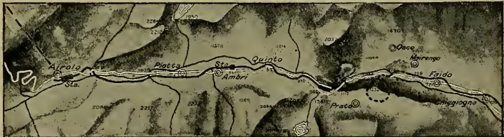
FIG. 39A.—Loop Tunnels of St. Gothard. Approach to the Great Tunnel from the South.
