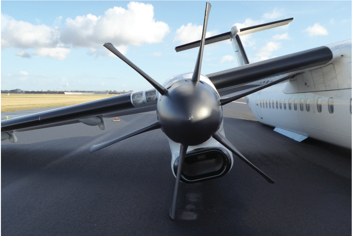
Figure 4: right-hand nacelle and MLG after occurrence. (source: Dutch Safety Board)
