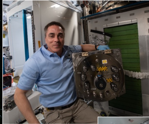
Left: Installation of the Urine Processor Assembly (UPA) Upgraded Distillation Assembly
