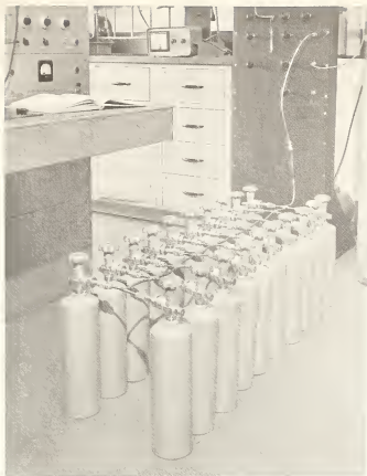
Figure 4. Filling twenty small cylinders from master mixture.
