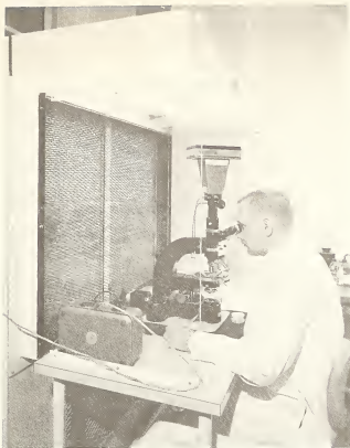
Figure 22. Laminar flow clean bench.
