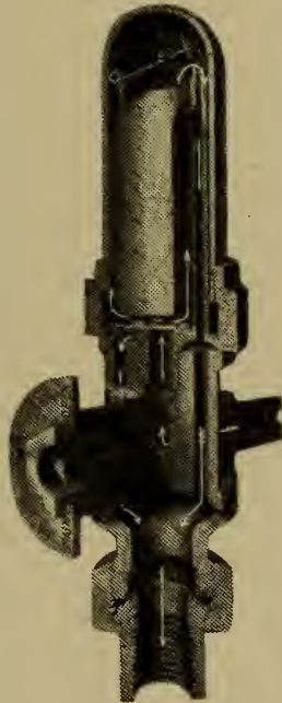
Figure 77. Air valve adapted to hot water work.
