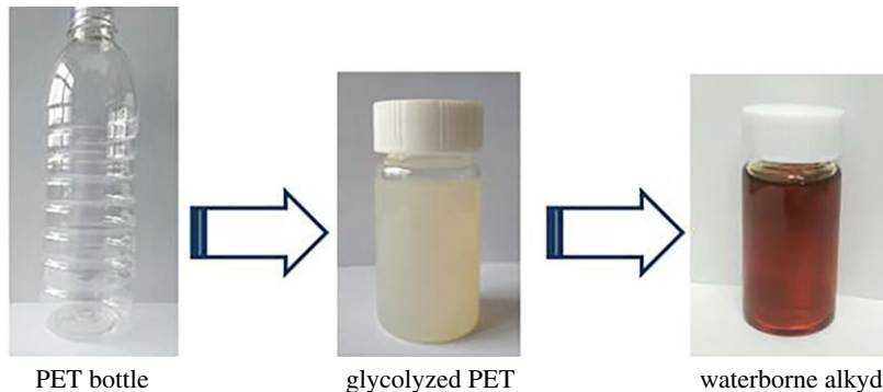
Figure 2. The appearances of the glycolyzed PET and waterborne alkyd.
