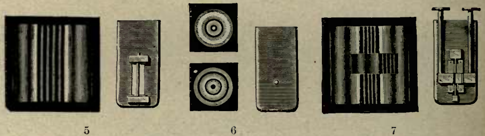
Diffraction Phenomena with narrow Apertures. Fig. 21. 1:3.
