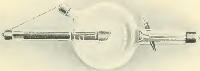
FIG. 31.—Heavy anode tube (Gundelach). Osmosis regulator. (Siemens.)
