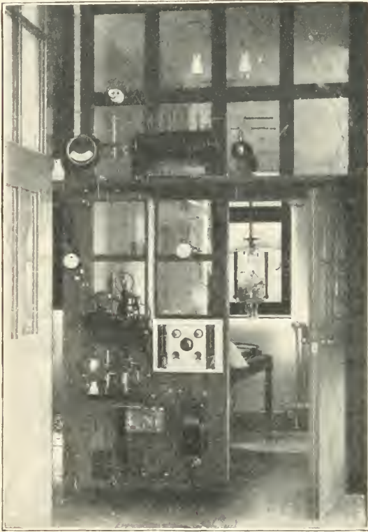
FIG. 185.—X-ray treatment cubicle. ( Archives of Röntgen Ray. ) Control apparatus arranged outside the cubicle.
