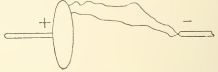
FIG. 37.—Connections of the X-ray tube to the coil, showing the appearance when the poles are reversed.
