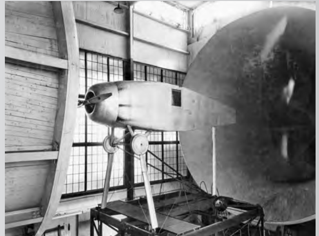
Section of aircraft tested for drag in Langley wind tunnel. (NASA image 1974-L-02730)
