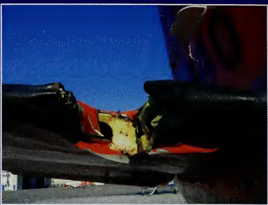
Figure 1 —Bird strikes affect both civil and military aircraft: this Navy plane collided with a single turkey vulture in Florida.
