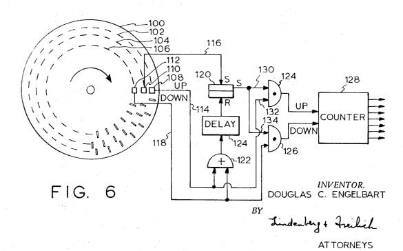
X-Y POSITION INDICATOR FOR A DISPLAY SYSTEM
