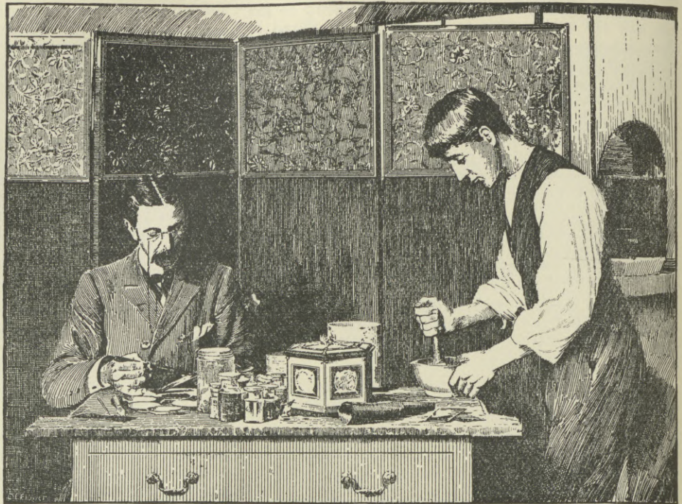
FIG. 1.—Laying enamel on a copper plate, and pulverizing enamel with a pestle and mortar.
