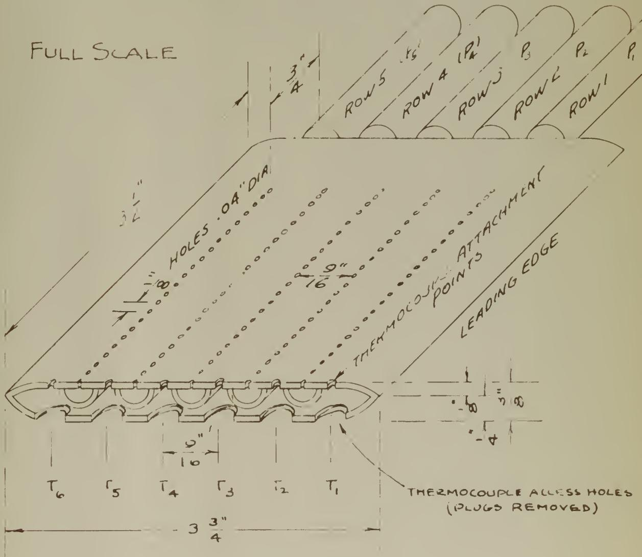
BLADE CROSS SECTION AT THERMOCOUPLE ATTACHMENT POINTS
