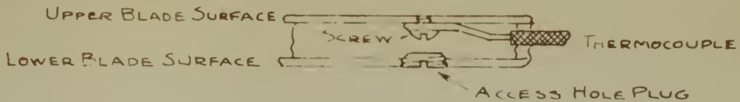
METHOD OF ATTACHING THERMOCOUPLE TO BLADE
