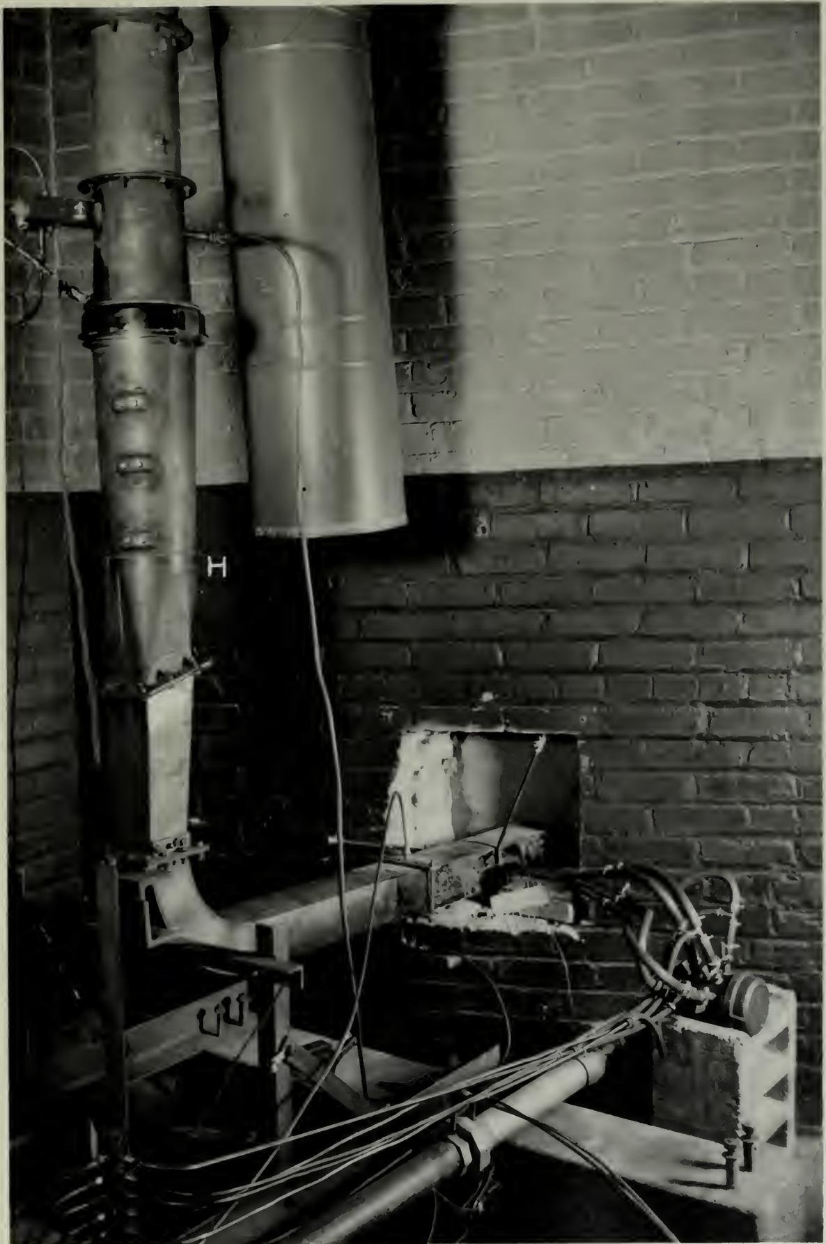
Figure 14 Burner and Test Section
