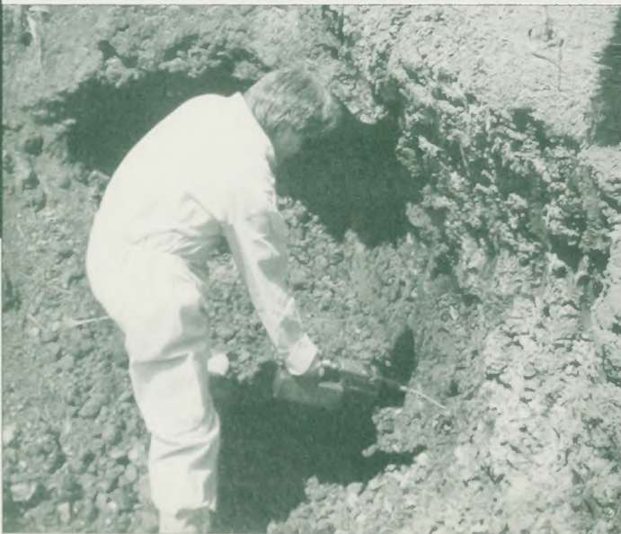
Field analysis for volatile organic vapors, using a photo ion detector (Cottonwood Field Office, Upper Columbia - Salmon Clearwater BLM District).
