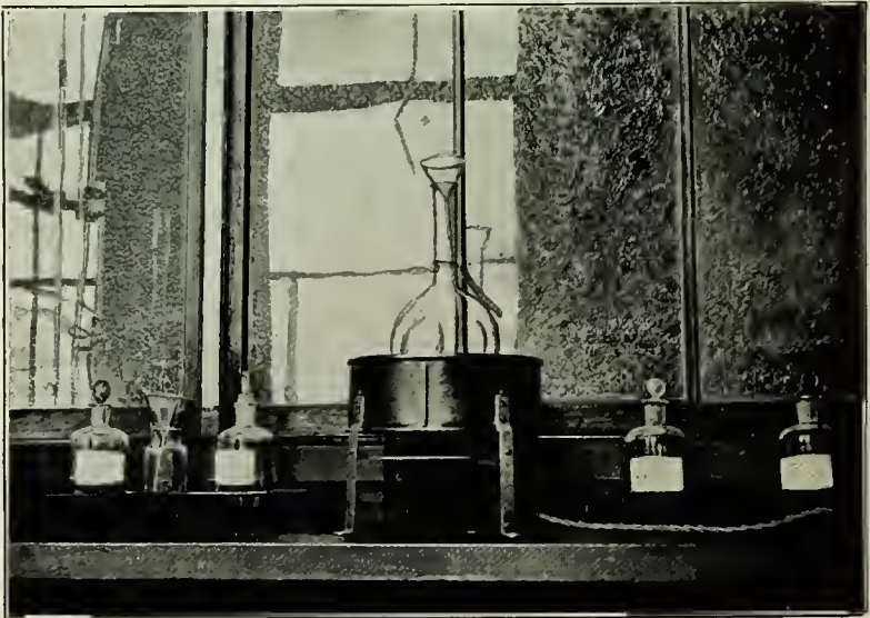
ELECTRIC FLASK HEATER IN USE IN LABORATORY FOR WATER ANALYSIS
