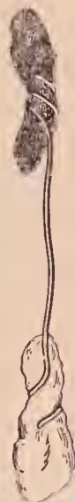
FIG. 36. — Wads of cotton and iron thread for studying the properties of chlorine
