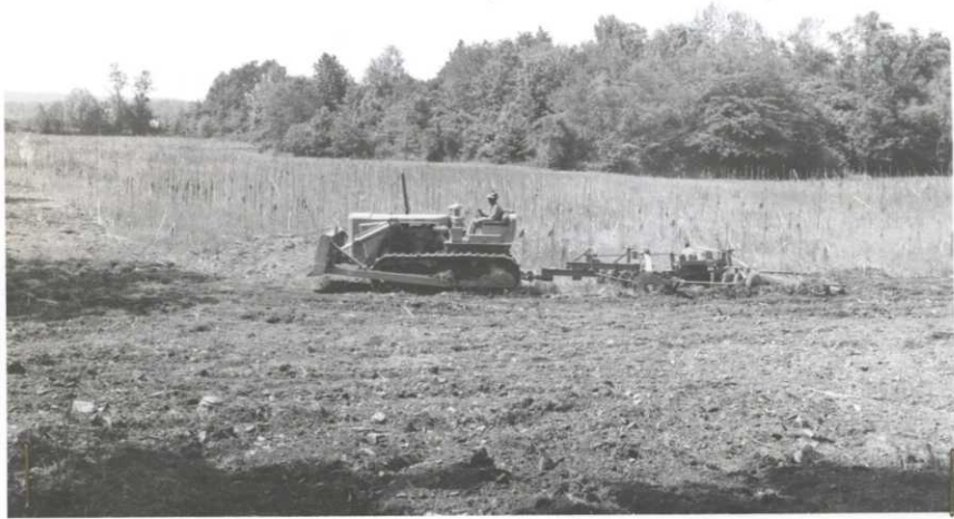
Cooperator Rochelle using D-6 tractor and Rome Harrow Plow M-20-28 to make seed bed in one operation. Duck River Refuge, May 1950.
