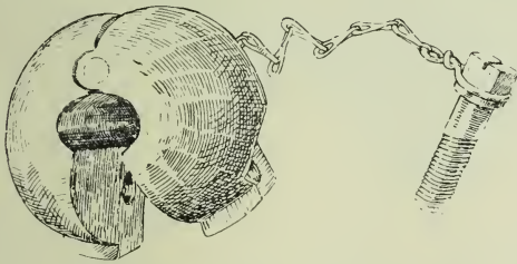
FIG. 33.—BRASS KNOB FOR TOW-NETS.
