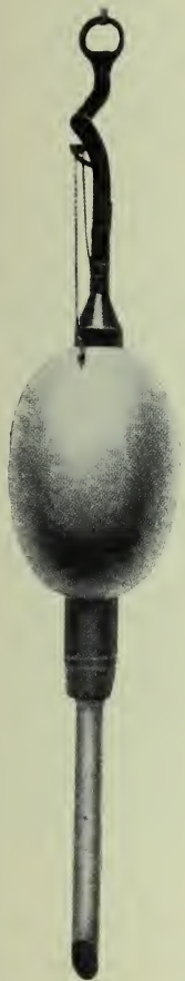
FIG. 6.—SIGSBEE'S SOUNDING-TUBE. (From Brennecke.)
