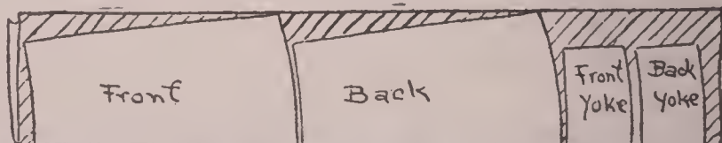
Fig. (33) Diagram showing yoke skirt pattern placed on the goods for cutting
