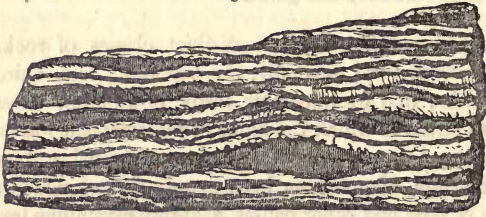
Fragment of gneiss, natural size : section made at right angles to the planes of foliation.
