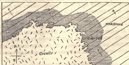
Altered zone of fossiliferous slate and limestone near granite. Christiania. The arrows indicate the dip, and the straight lines the strike, of the beds.
