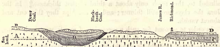
Section showing the geological position of the James River, or East Virginian Coal-field.
