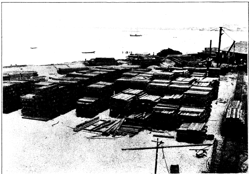
Piled ties, bridge, and car timber, ready for treatment in plant A NEW INDUSTRY IN THE PHILIPPINES
