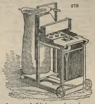
lent. By turning a keeper fixed to the scale, one end of it is opened, turning on a cylindrical hinge at the top, and the contents speedily discharged. These balances may be made of any size required, either to suit the purposes of the farm, or the household. Their simplicity secures them equally against expense of manufacture, and the risk of going wrong when in use. One weight only is required, the value of which, as a counterpoise, depends on its distance from the centre of motion; and it
