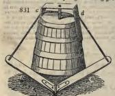
removed, the beaters (b) may be taken out at pleasure by withdrawing the spindle (c) to admit the removal of the butter, or the cleaning and scalding of the churn.
