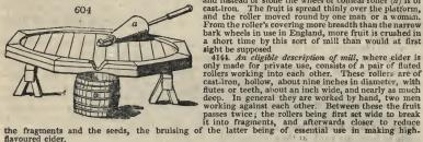
4143. A cider-mill in use in the south of France (fig. 604) is worked on a circular platform of boards, and instead of stone the wheel or coulcal roller (a) is of cast-iron. The fruit is spread thinly over the platform, and the roller moved round by one man or a woman. From the roller's covering more breadth than the narrow bark wheels in use in England, more fruit is crushed in a short time by this sort of mill than would at first sight be supposed
