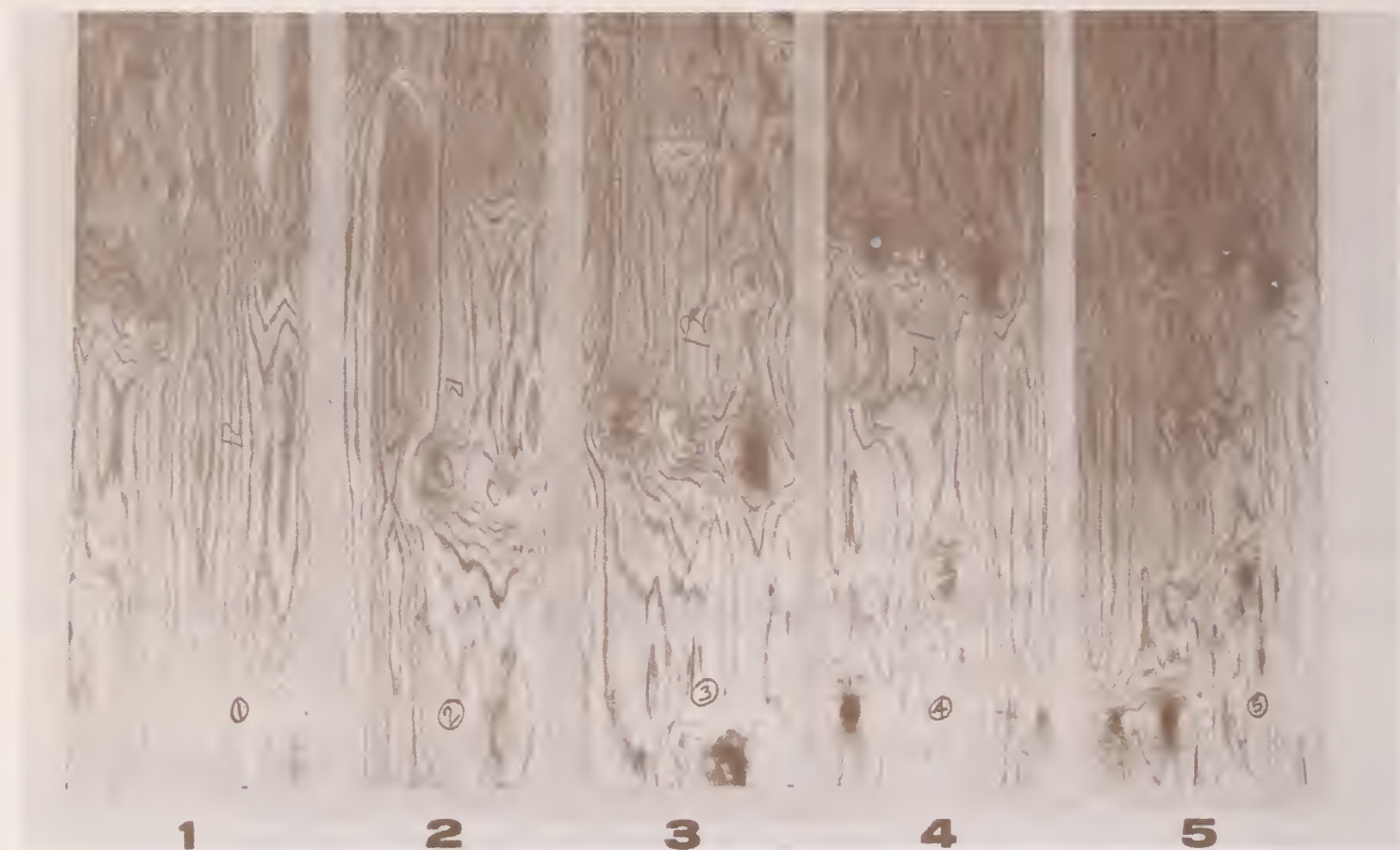
Figure 20. Veneers of red oak logs are shown in decreasing order of quality: 1-Face; 2-Veneer next to face; 3-Third veneer; 4-Fourth veneer; and 5-Fifth or the innermost veneer. Mississippi State University, 3626.
