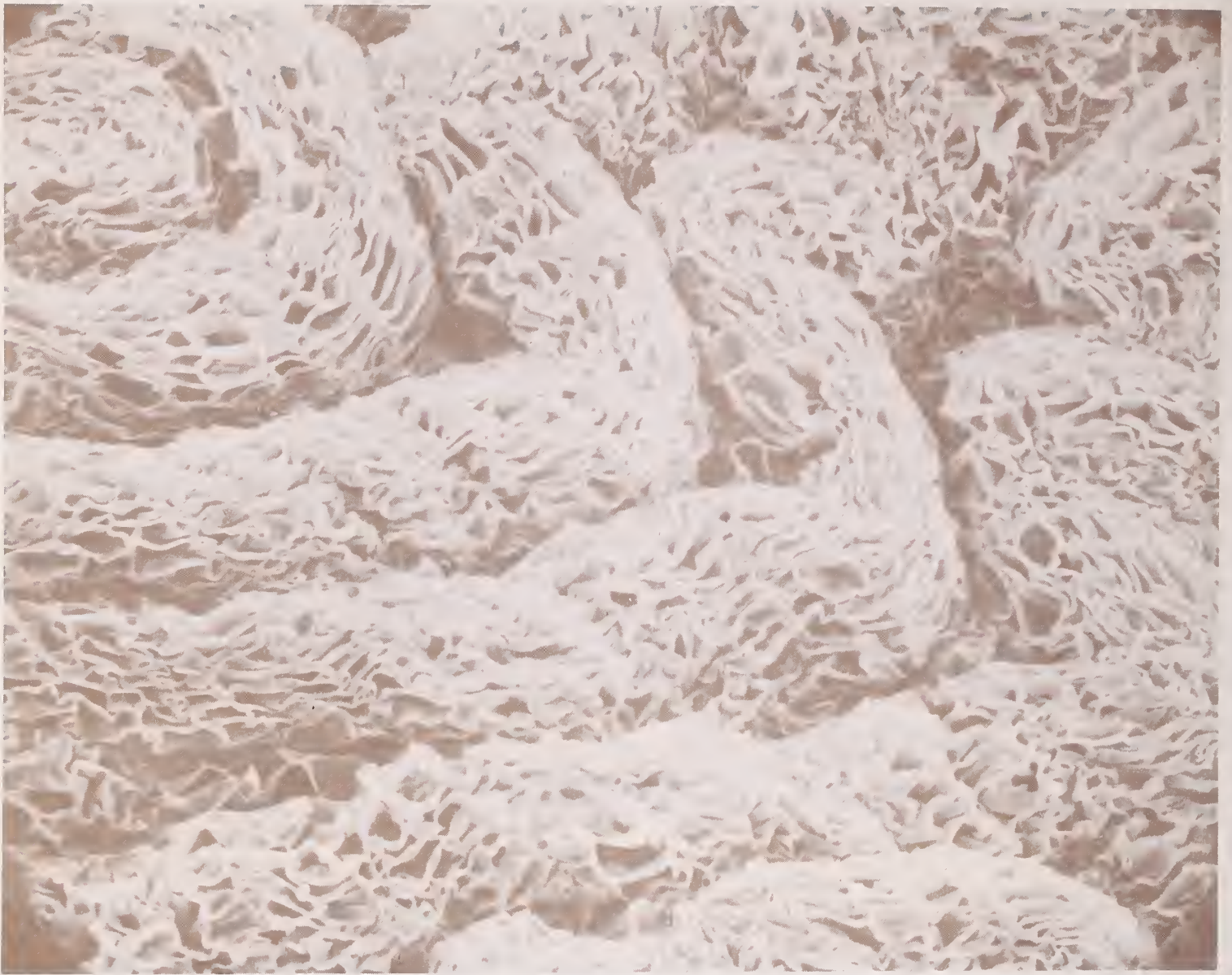
Figure 21. This scanning electron micrograph of Douglas-fir bark reveals the altered structure of a cork particle after it has been treated with solvent. Oregon State University, F-879.
