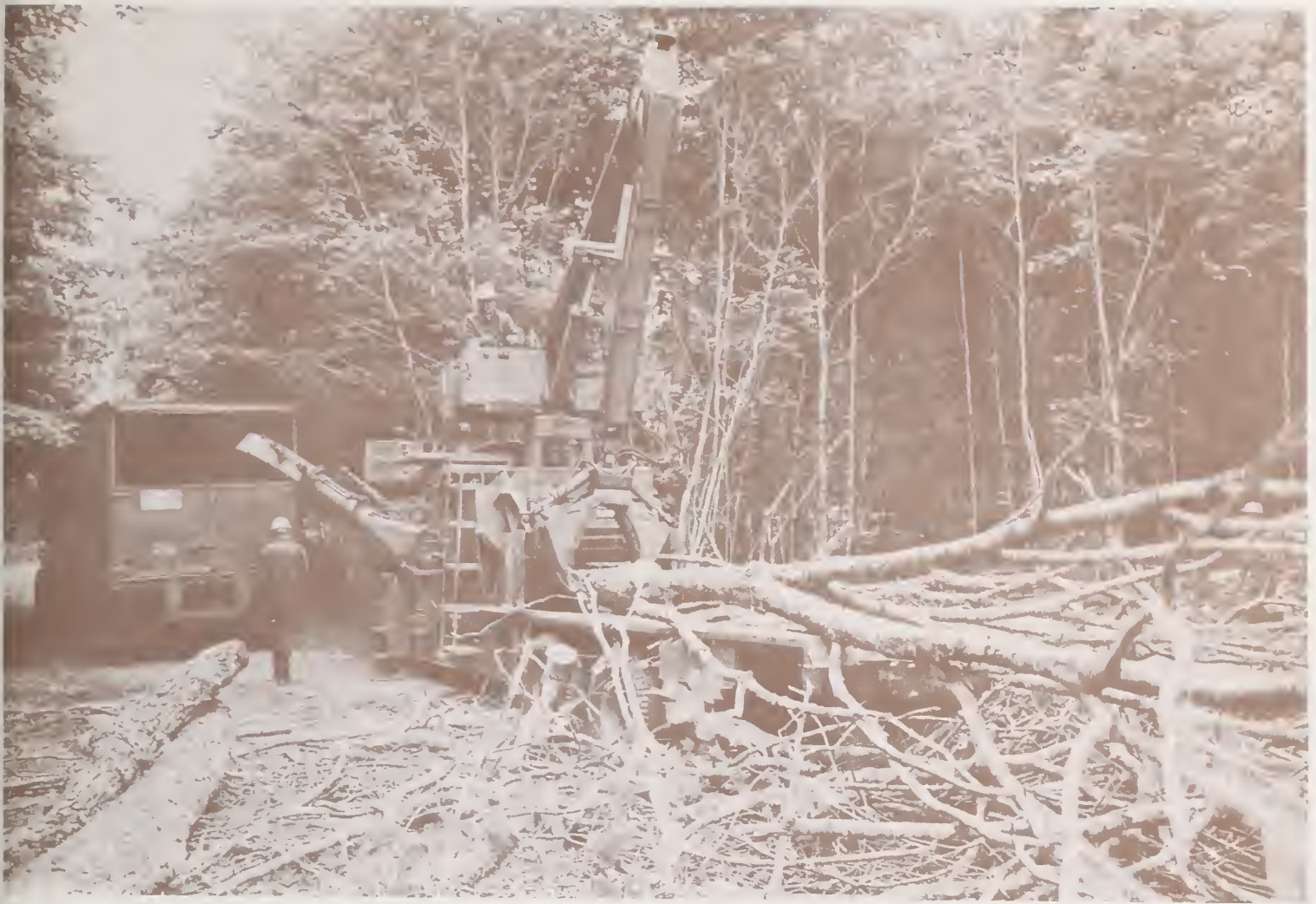
Figure 17. Hardwood logging residue of various shapes and sizes is easily reduced to chips by the chip harvester. Chips can be blown directly into vans (at left in photograph), or they can be screened on the site with a portable screen. Michigan Technological University, 2-3310.
