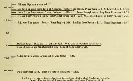
It is evident that in the city of New York there must be much confusion resulting from the use of so many datums, and it is possible that the confusion in the elevations and the datums may involve the city in much extra expense on engineering work, due to errors which must inevitably be made in interpreting the leveling data.
