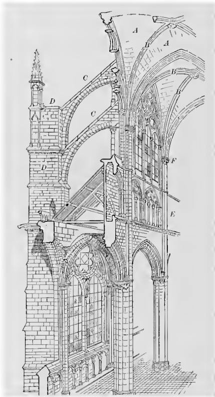
FIG. 183. CROSS SECTION OF AMIENS CATHEDRAL
