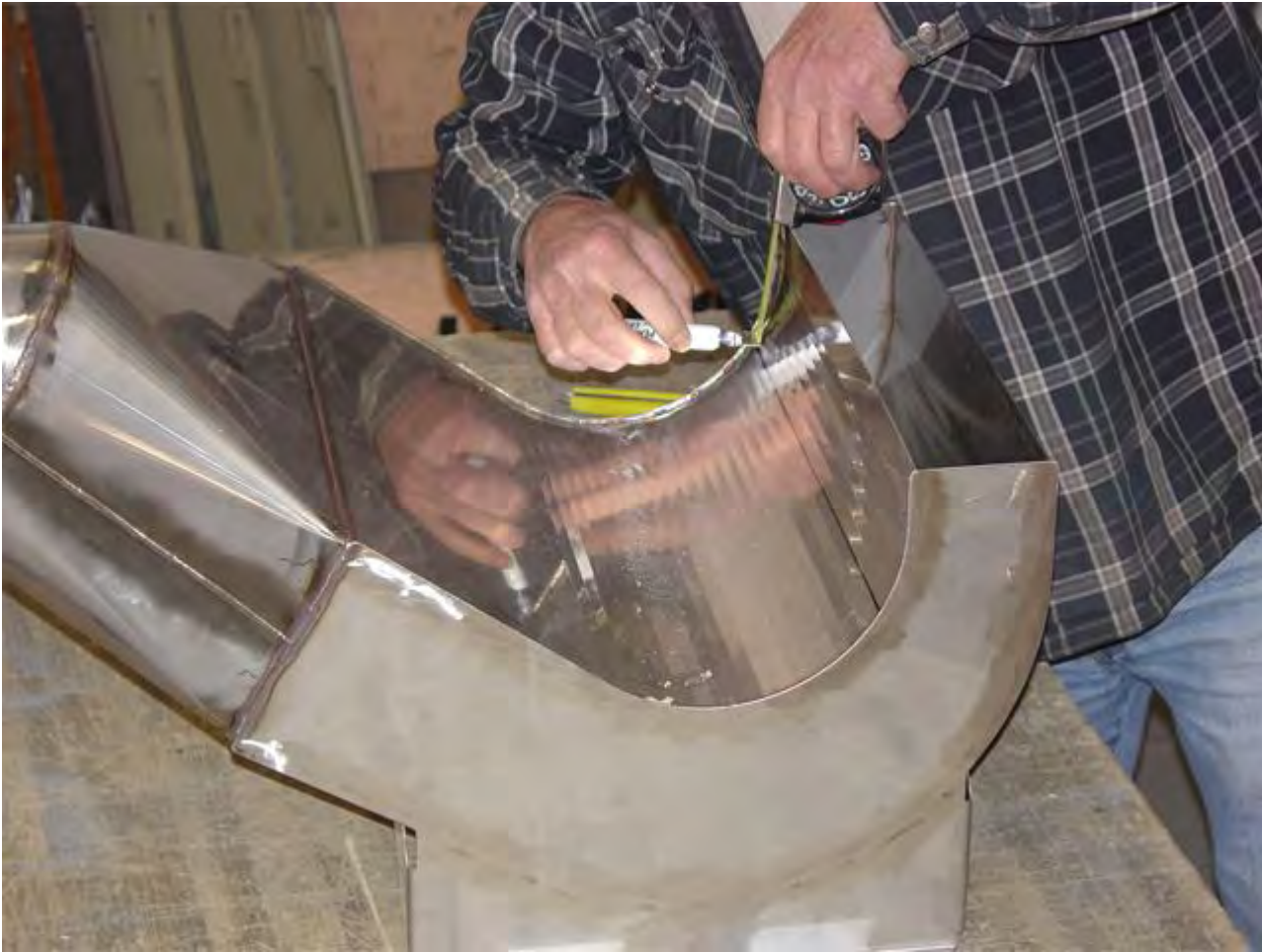
Figure 13. Measuring the Plenum.
