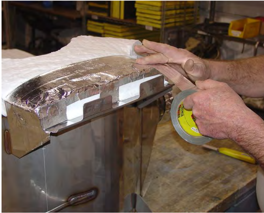
Figure 18. Wrapping of the Plenum.
