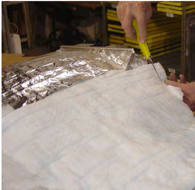
Figure 26. Trimming Insulation from Plenum (Sheet 1 of 2).
