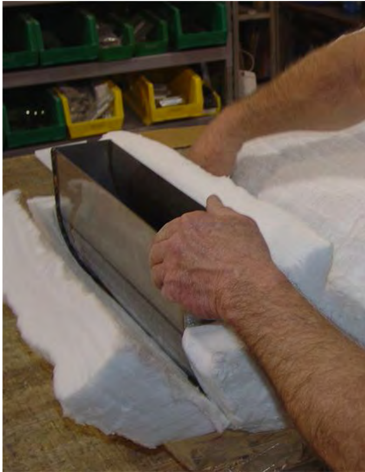
Figure 30. Snugging Insulation into the Bend (Sheet 2 of 2).
