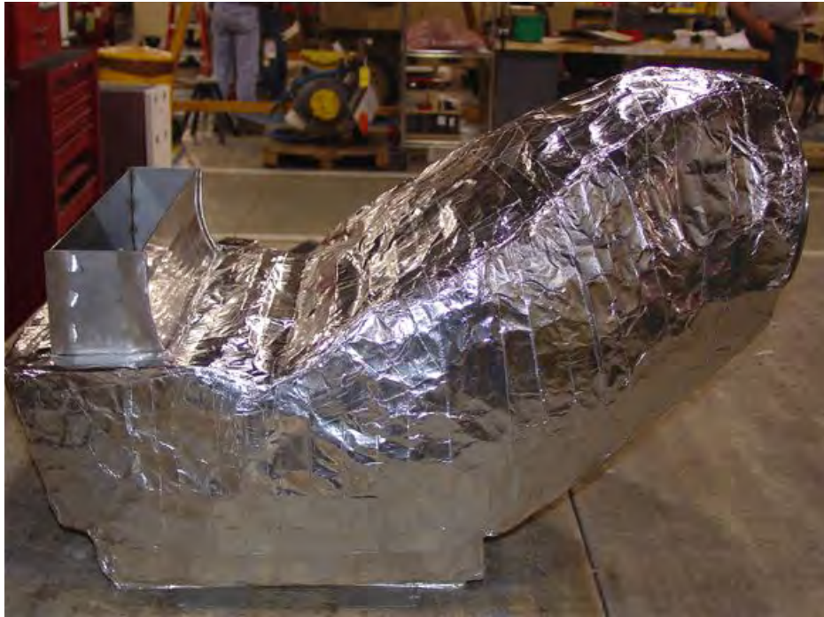
Figure 40. Bottom and Top View of Completed Insulation Wrap (Sheet 2 of 2).
