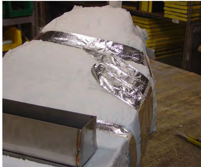
Figure 33. Taping the Top of the Unit (Sheet 1 of 2).
