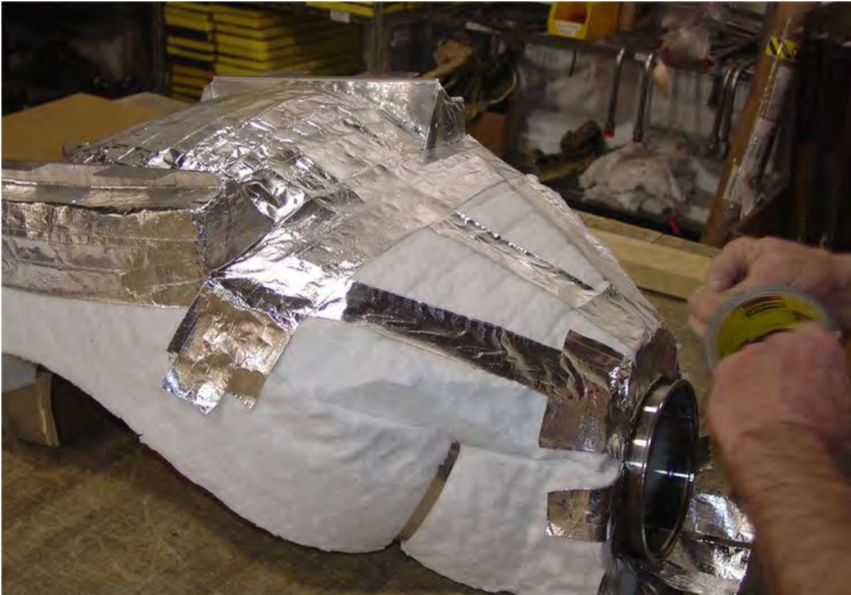
Figure 29. Insulating the Top Snug (Sheet 1 of 2).
