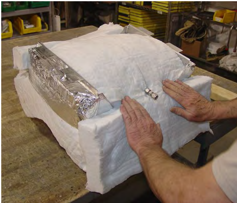
Figure 22. Placing Insulation on the Bottom of the Plenum Showing the Extension Tube.
