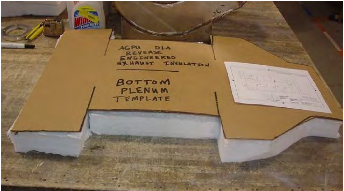
Figure 11. Plenum Template (Sheet 3 of 3).
