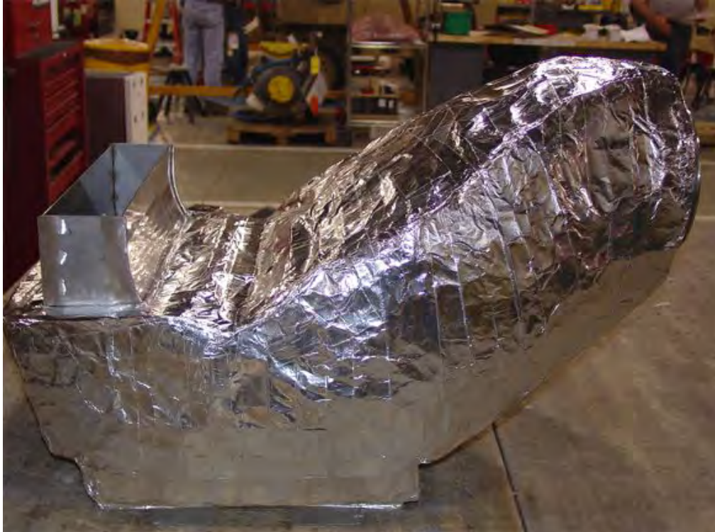
Figure 6. Plenum Insulation Wrapping Instructions.
