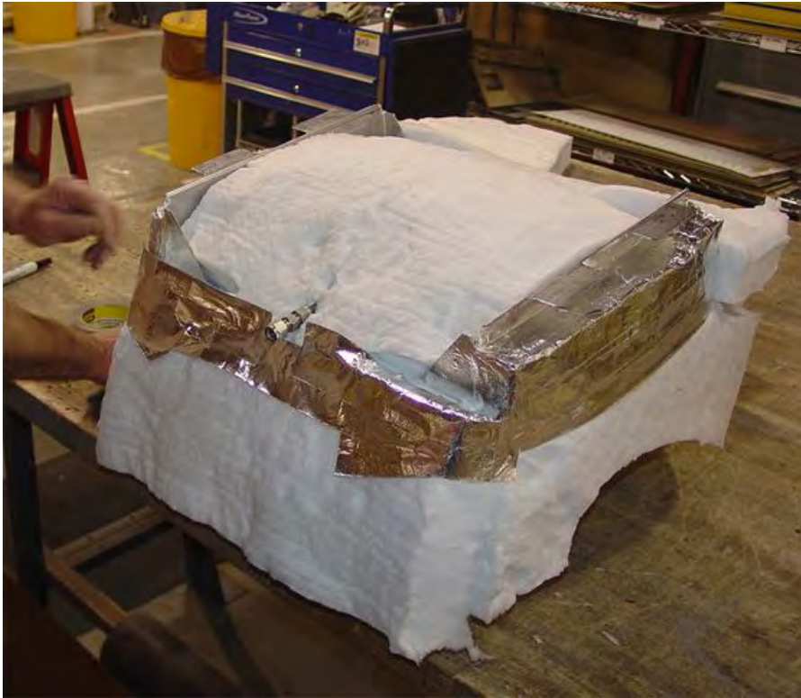
Figure 24. Taping Down the Insulation (Sheet 1 of 2).
