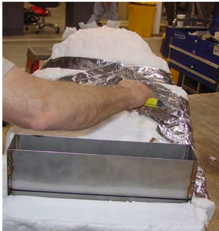
Figure 33. Taping the Top of the Unit (Sheet 2 of 2).
