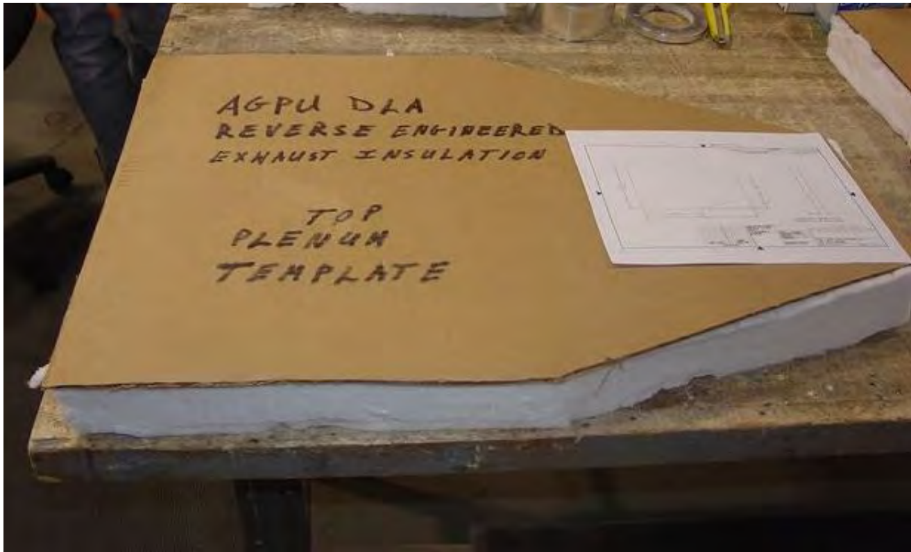
Figure 11. Plenum Template (Sheet 1 of 3).
