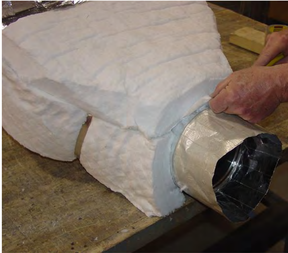
Figure 27. Trimming Insulation Around the Inlet (Sheet 2 of 2).
