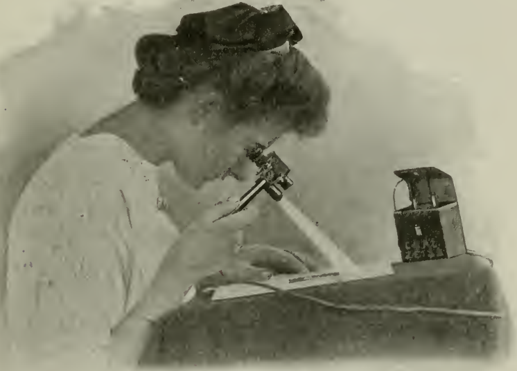
Monocular Telescopic Magnifier with Illuminating Attachment, showing manner of using the apparatus.
