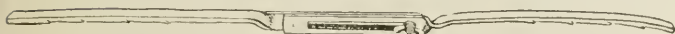
FIG. 3. Fig. 3. To be used on under side of leg when extra strength is required. Arms 9"x24"x3-16". Cross bars 4" long.
