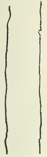
FIG. 4.—A tracing by camera lucida of the margins of an ink line drawn by a pen fixed to a ruling machine. It is enlarged 60 diameters. There is an absence of the irregularities always found in the margins of ink lines made by the human hand.
