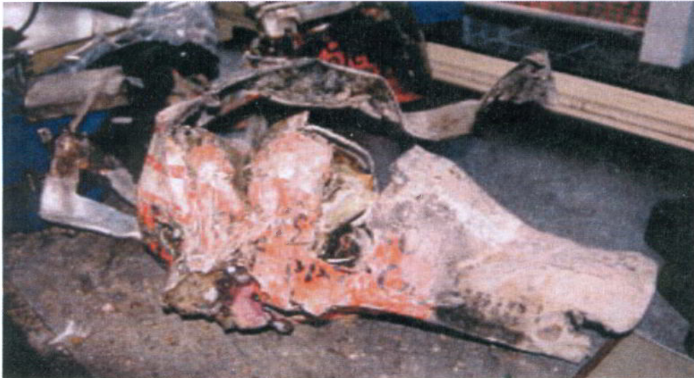
FDR unit (crash protected enclosure normally located on right hand side (front of unit))
