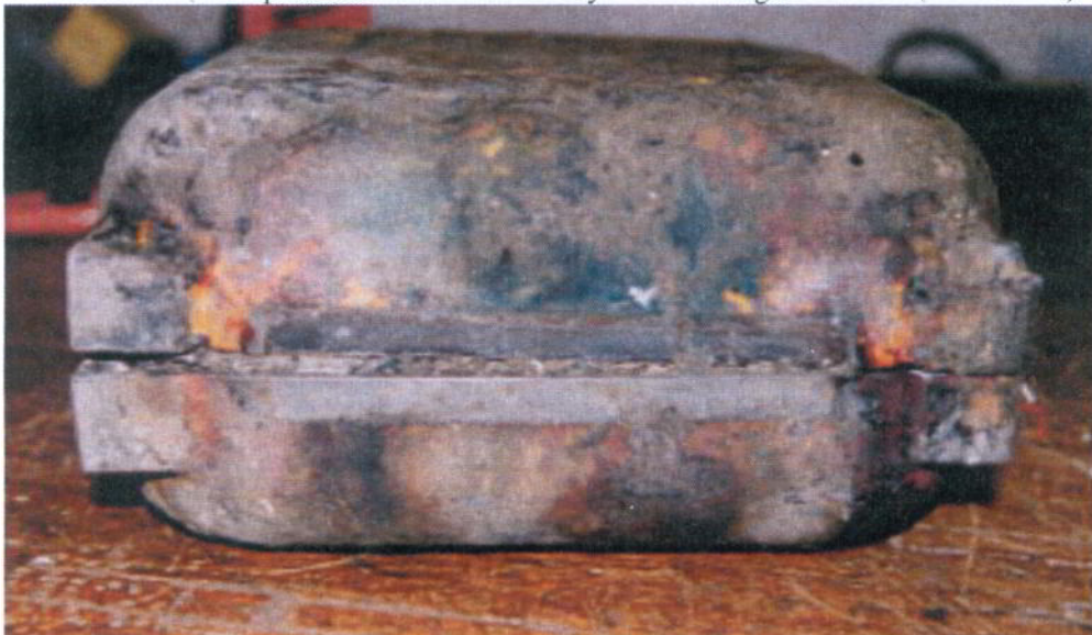
Crash Protected enclosure (showing separation of the two halves)
