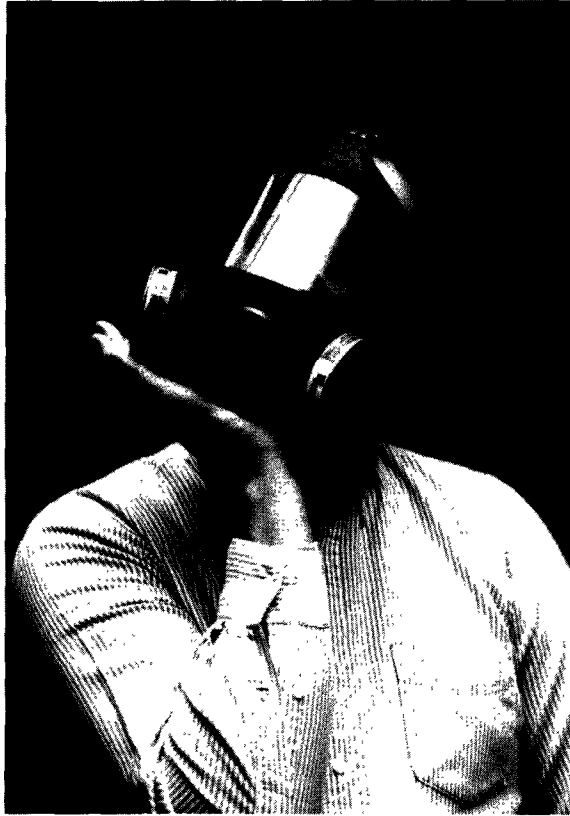
Photograph 8. Positive pressure test; blocking exhalation valve.
