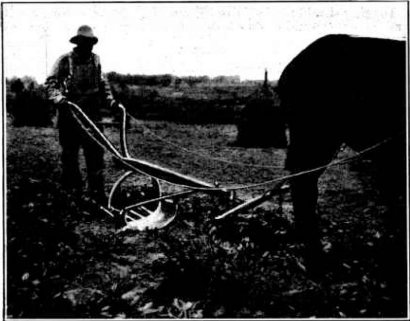
FIGURE 8.—A simple and effective peanut digger made by a local blacksmith
