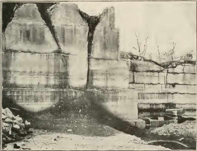
Fig. 7. A quarry face in the Hunter valley region, Bloomington, showing joints widely opened by solution.
