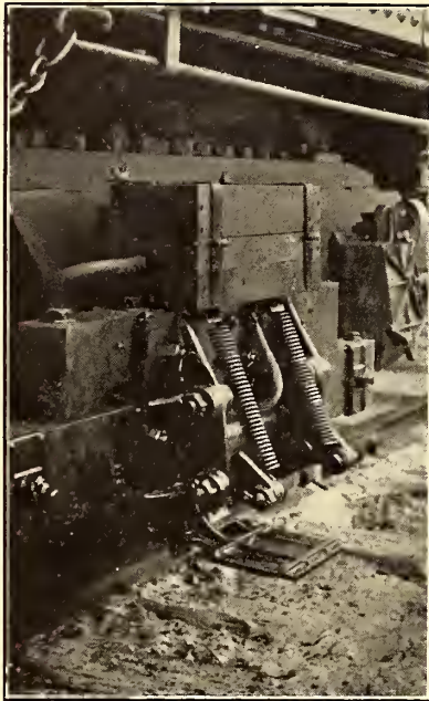
Inner Position Outer Position FIG. 15.—ADJUSTABLE THIRD-RAIL SHOE IN TWO POSITIONS
