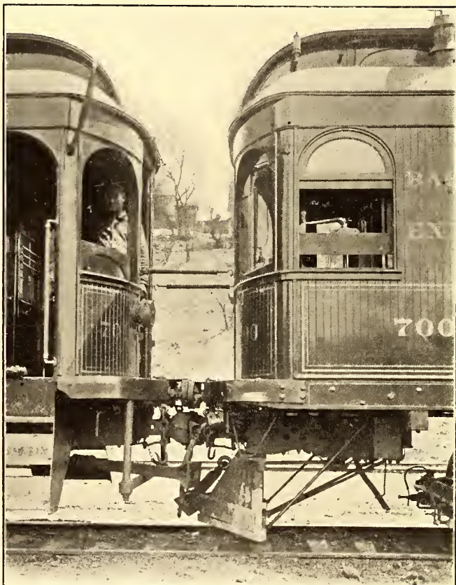
MANNER OF COUPLING CARS, THE SPRING BUFFERS AND PROTECTING ARM RAIL PERMITTING PASSAGE BETWEEN THE CARS
