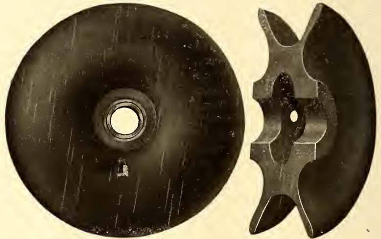
SIDE VIEW AND SECTION OF TROLLEY WHEEL
