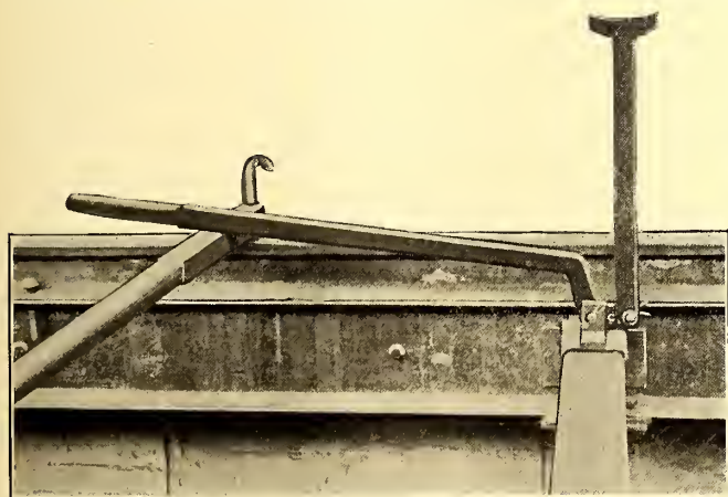
FIG. 4.—APPARATUS FOR TESTING ARMATURE BEARINGS
