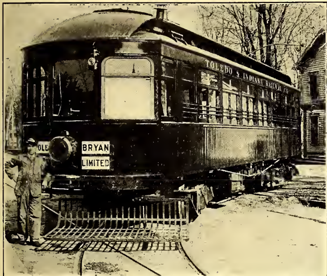
HEAD-ON VIEW OF CAR, SHOWING FENDER CONFORMING TO CURVATURE OF TRACK
