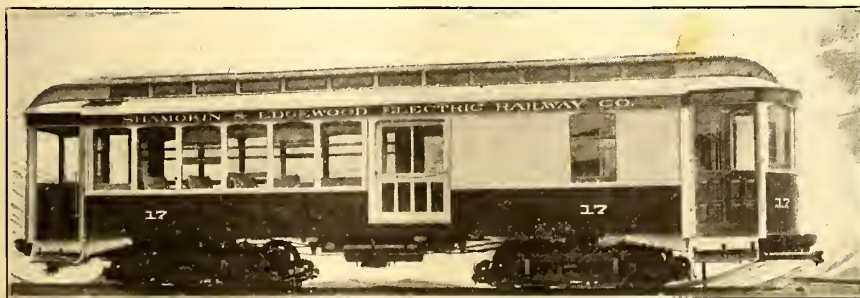
COMBINATION PASSENGER AND BAGGAGE CAR FOR THE SHAMOKIN & EDGEWOOD ELECTRIC RAILWAY COMPANY
