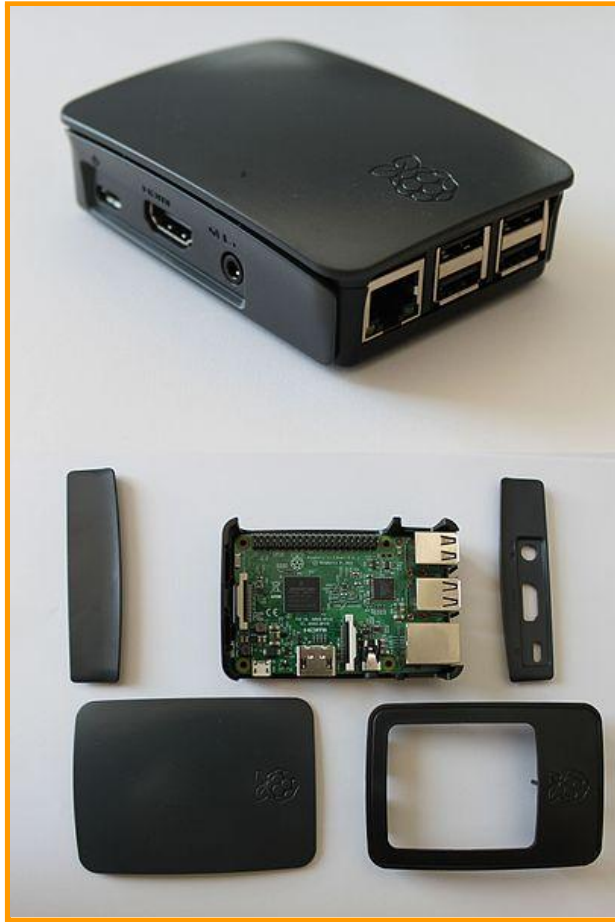
The black protective case of the Raspberry Pi 3. Top: the fully set-up case. Bottom: the different elements of the case. Author: Jose.gil. CC by sa 4.0
