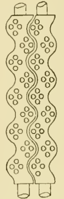
END SINUOUS PIECES AND ARRANGEMENT OF TUBES ON AN ENLARGED SCALE
