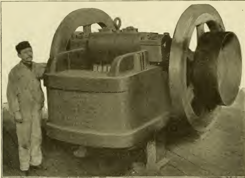
NEW STONE-BREAKING MACHINE FOR ROAD-MAKING.
