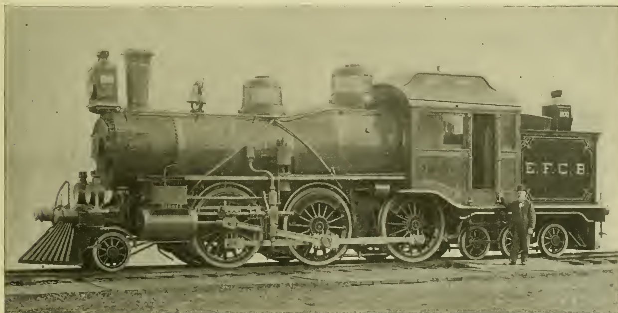
SUBURBAN LOCOMOTIVE FOR THE CENTRAL RAILWAY OF BRAZIL. BUILT BY THE BROOKS LOCOMOTIVE WORKS, DUNKIRK, N. Y.
