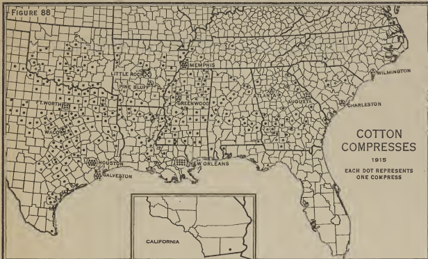
Figure 88.—Compresses are located at large markets and points at which cotton is collected from the smaller markets to be shipped long distances. In the West, where most of the cotton is exported or shipped to New England, they are numerous; while in the East, where much cotton is consumed in the local mills, they are few.
