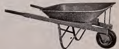
Lightest practical full-sized utility barrow on the market, yet sturdy enough to carry a load of 250 lbs. Size of tray 32 \times 29 inches, capacity 3 cubic feet, weight 35 lbs. Channel steel legs, hardwood handles. Wheel cadmium plated steel disc type, tire 10 \times 2\frac{3}{4} inches, donut single tube cord. Price, $7.75.
