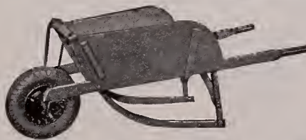
Vaughan's Greenhouse. Made especially for use in greenhouses between the benches. Dimensions are as follows: Box, 14 in. wide at wheel end; 16 in. wide at handle end; 12 in. deep. The bottom of the box is matched and glued together, and there is no crack against which a shovel might run. The wheel is of steel, 17 inches high, with 2\frac{1}{2} -inch thread; the axle is 15 inches wide. Made of the best material. Legs reinforced, spread at handles at hand-hold 20 inches, which is extreme width of barrow. Price, each, $9.25.
