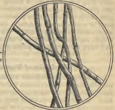
The annexed engraving represents the appearance of the ordinary flax fibre, as seen under the microscope.
