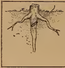
The dynamite charge should be placed below the depth of plowing and at the center of greatest resistance
