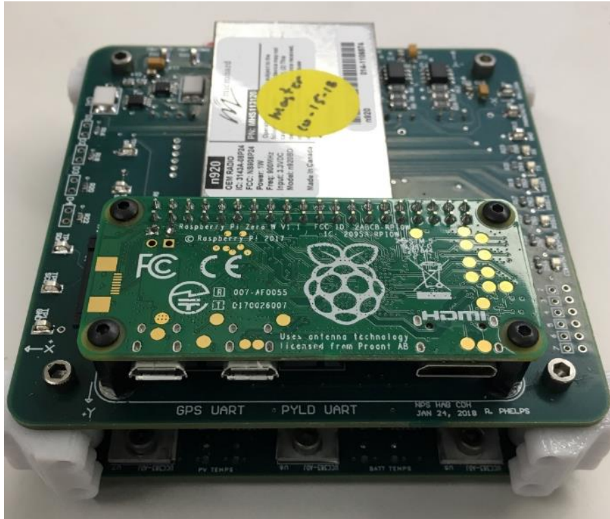
Figure 24. Com-Cube C&DH and EPS Printed Circuit Boards.
