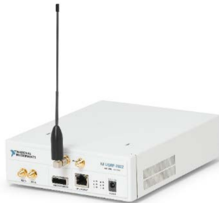
Figure 63. National Instruments USRP-2922 SDR [54].
