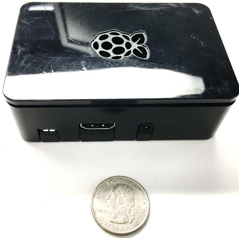
Figure 16. Raspberry Pi 3 Model B with Commercial Vendor Enclosure Box Compared to a Coin.
