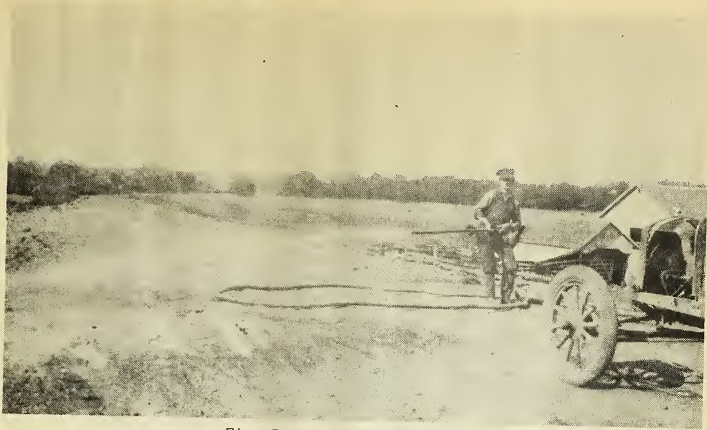
Fig. 3. - Sixty pounds per square inch pressure or more should be maintained on the 1/2-inch nozzle of the jet
