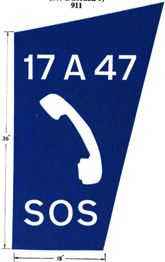
Side of emergency telephone box (See Direction 9) 914
