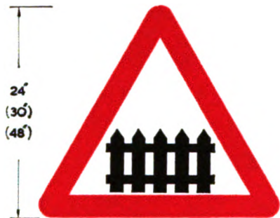
Level crossing with gate or barrier 537
