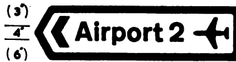
Direction to airport with mileage Permitted variant: The name of the airport may be included 733
