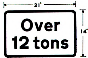
Plate for use with sign in diagram 630 Note: The figure quoted relates to laden weight (See Directions 6, 11 and 12) 631
