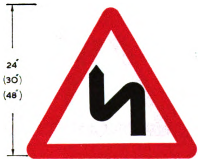
Double bend, first to the left Permitted variant: The symbol may be reversed 513
