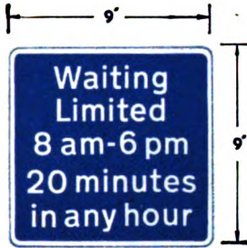
Plate showing hours during which waiting is limited (See Directions 6, 13 and 28) 641
