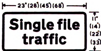
Convergence of traffic to single file Plate for use with signs in diagrams 516 and 517 (See Direction 12) 518
