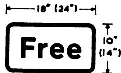
Plate for use with sign in diagram 801 indicating a free car park Permitted variant: The legend may be varied to accord with any conditions imposed on the use of the car park (See Direction 12) 805
