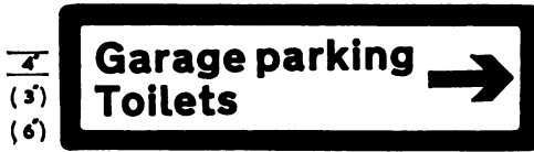
Direction from junction ahead to local places 731
