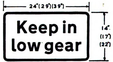
Continued existence of very steep hill Plate for use with signs in diagrams 512, 513, 523 and 524 (See Direction 12) 526
