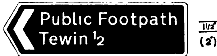
Footpath direction sign with mileage to place indicated Permitted variant: Bridlepath or Bridleway may be substituted for Public Footpath 740
