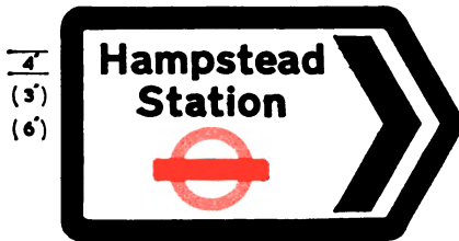
Direction to London Transport station 734
