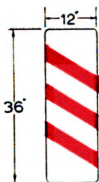
Concealed level crossing ahead 539
