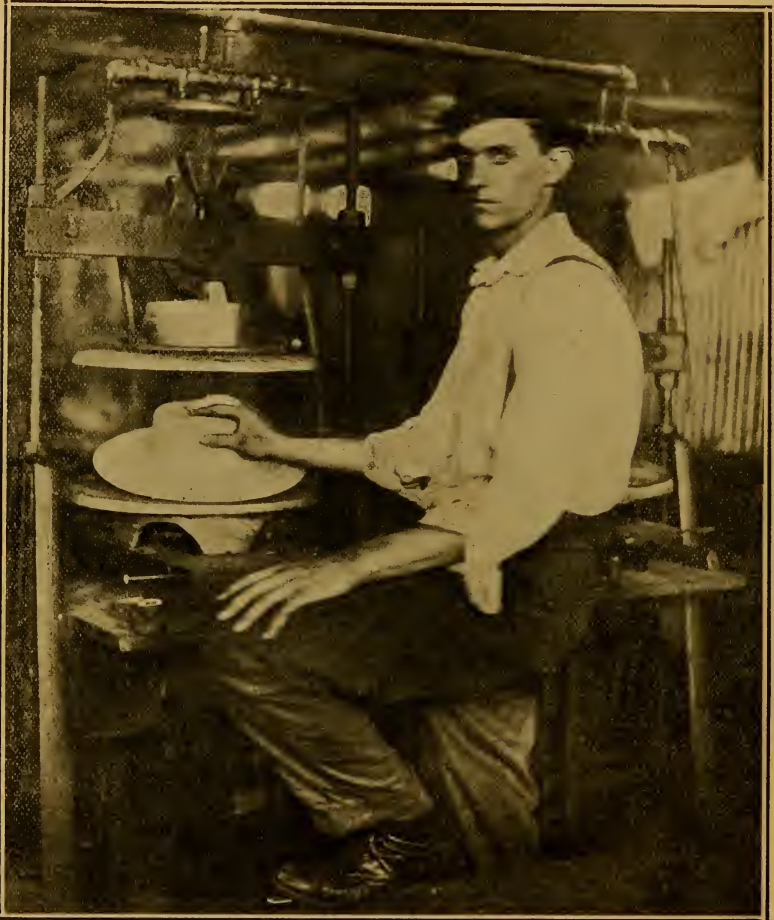
A STEAMING PROCESS SOFTENS THE SHAPE AND IT IS PUT IN AN IMMENSE MOULDER
