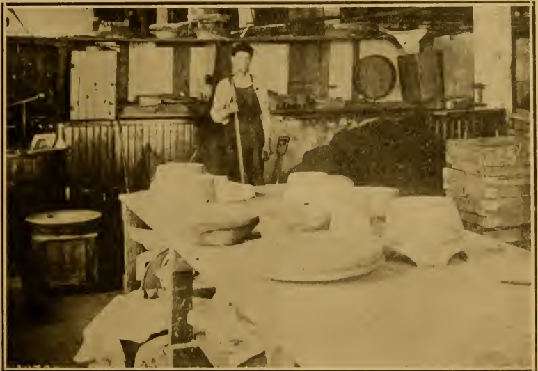
MOULDING ROOM, WHERE PLASTER-OF-PARIS MOULDS ARE MADE OF THE SEASON'S "PATTERN HATS"
